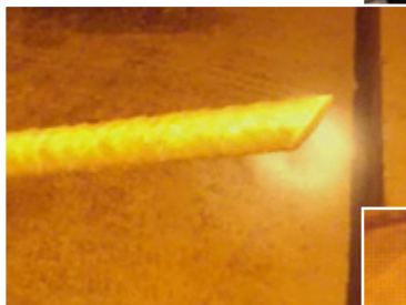
45° fiberglass end for easy resin penetration
